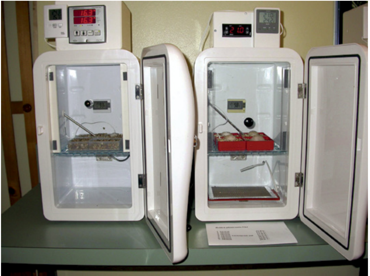
Several small incubators were constructed for egg incubation, each equipped with a thermostat capable of allowing a nighttime drop in temperature.
